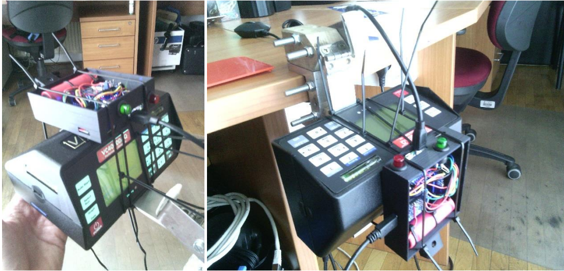
Fig. 8 Tilt device for testing the measuring values and triggering (left in horizontal position, right in vertical position)
